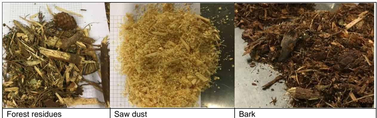
Figure 2. Pictures of the tested biofuels
