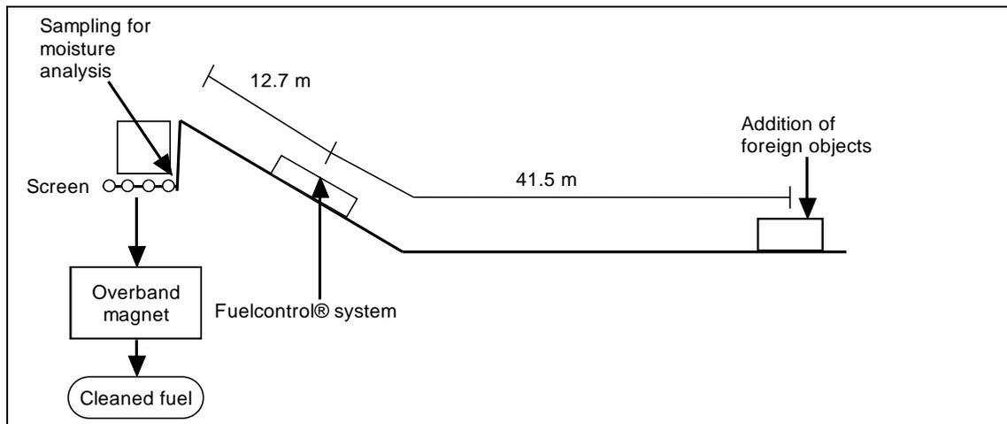
Figure 1. Positions for sampling, addition of foreign objects and FUELCONTROL® system
