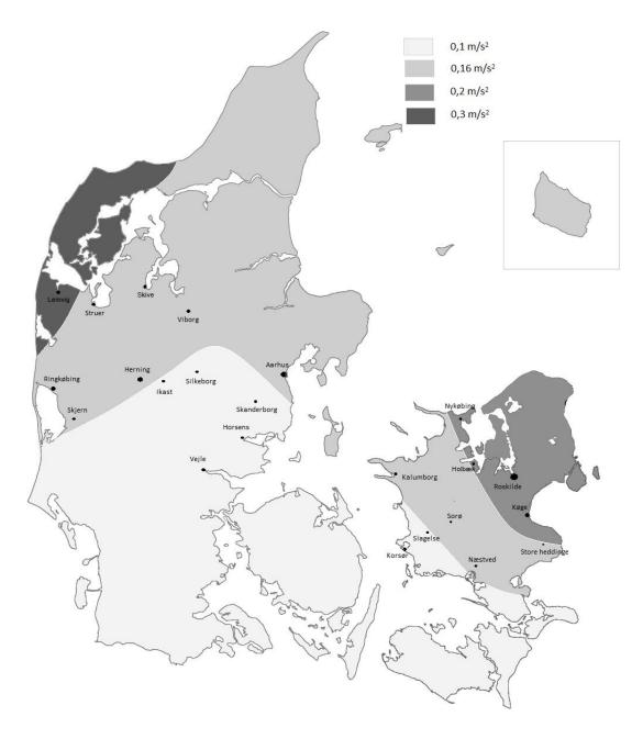
Figure D.2 DK NA: Values of design ground acceleration,  $a_{\rm g}$  The values are given in m/s<sub>2</sub>.
